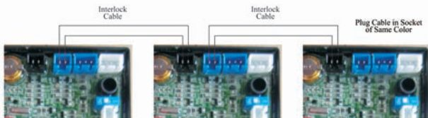
Figure 3-9 Network System Wiring with Interlock Cable
